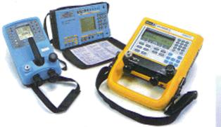
Left: DPI 610 Field Portable Pressure Calibrator Centre: TRX-II Portable Documenting Calibrator Right: DPI 605 Precision Portable Pressure Calibrator Inset: LP Series of Low Pressure Sensors
