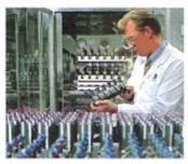
Computerised testing and calibration of pressure transducers.
